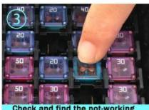
Check and find the not-working fuse and replace it.
