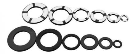
Strontium titanate varistor is a symmetrical varistor made of strontium titanate electronic ceramics sintered at high temperature. It has excellent voltage and current nonlinear characteristics and high capacitance, can suppress surge voltage, and is particularly suitable as a carbon brush protection and spark elimination element for micro motors.
